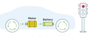
Energy is **reclaimed and stored** during braking, deceleration or coasting downhill.
