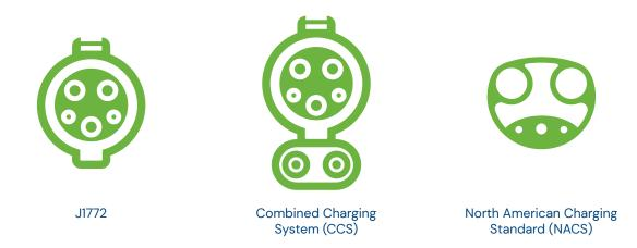
In the pioneer days of electric vehicles, *every* manufacturer had a proprietary plug. Needless to say, things were a little plugged up. Fortunately, the frontier has been (largely) settled. Here in the United States, manufacturers are circling the wagons around a <u>couple</u> <u>of different types of plugs</u>.
