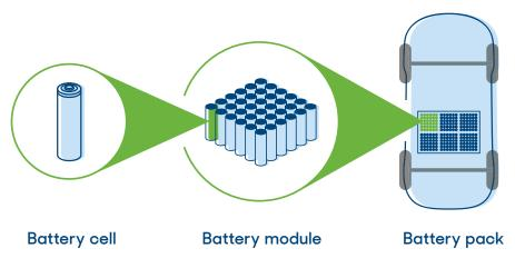
**Battery pack:** A group of battery modules. An EV's battery is where the electricity that powers your car is stored. Think of it as the fuel in your EV's "tank."
