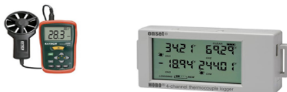
Figure 2: (Left) Anemometer, (Right) Thermocouple Logger for Space Temperatures
